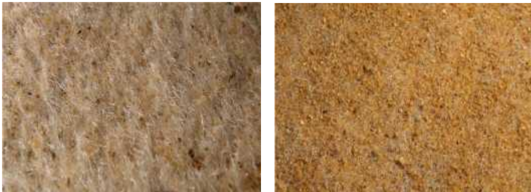
Fig. 8.1 Sand- fibre adhesion in GCL-River sand interface tested dry (left) and tested with 25% water content (right)
