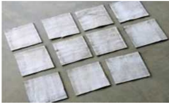
Fig. 3. The cut-out specimens of GCL
