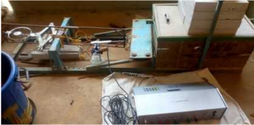
Fig. 1. Pullout test setup
