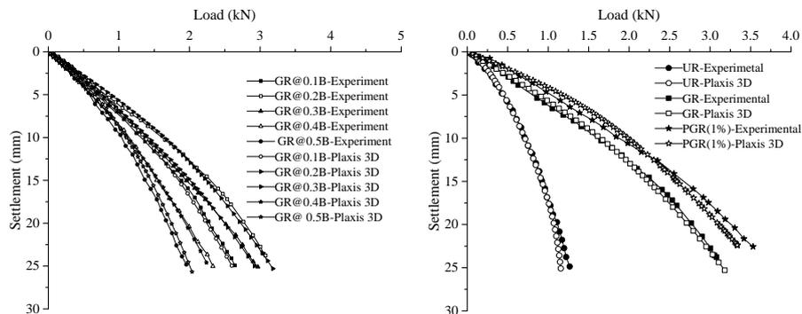
**Fig. 6.** Comparison of experimental and numerical studies.
