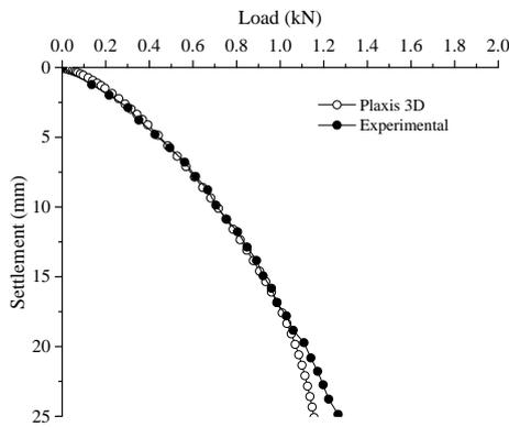
**Fig. 4.** Validation of Numerical study with the experimental data for unreinforced sand
