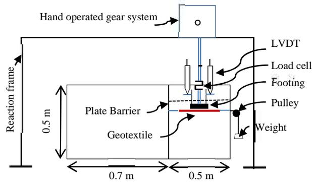
**Fig. 1.** Schematic diagram of the test set up
