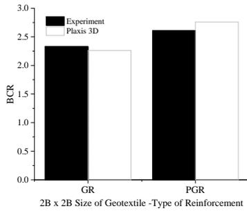
**Fig. 8.** BCR comparison for GR and PGR sand for numerical and experimental analysis.
