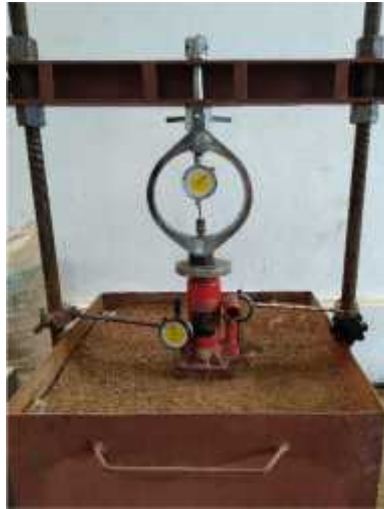
Fig. 3. Plate load test set-up
