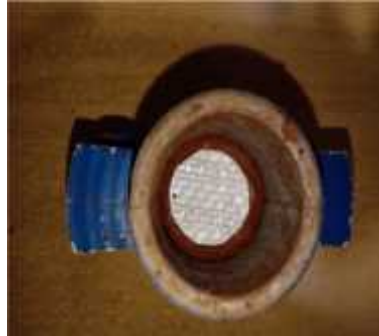
Fig. 3. Sample preparation with one layer of geotextile layer
