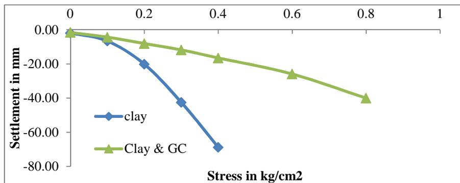
**Fig. 3** Comparison of Settlement at the end of 90 % consolidation with respect to Stress**Table 2.** Settlement at end of 90% consolidation (20160 minutes) and improvement factor (IF) for each stress level
