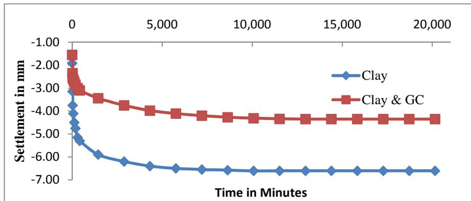
Fig. 2(b) Time vs settlement under sustained stress of  $0.1 \text{ kg/cm}^2$
