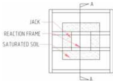
**Fig. 1(a)** Plan showing the loading frame.
