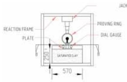
**Fig. 1(b)** Section A-A
