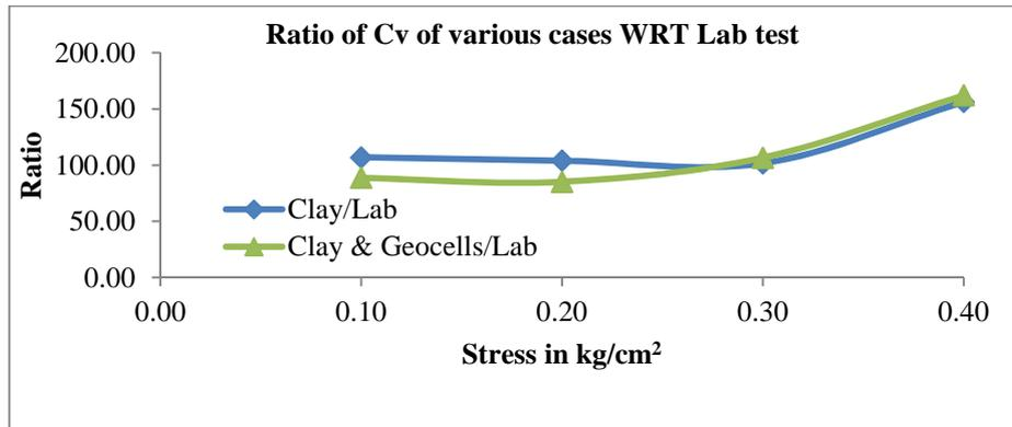
Fig. 11 Coefficient of consolidation of various cases WRT Lab
