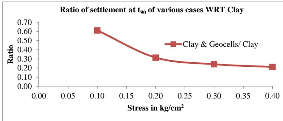
Fig. 8. Ratio of settlement at  $t_{90}$  of various cases WRT Clay
