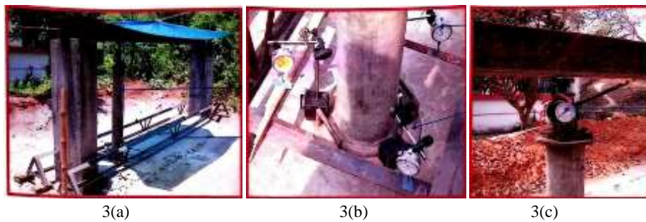
Fig. 3. Plate load test set up: (a) complete loading arrangement (b) dial gauge set up (c) hydraulic jack
