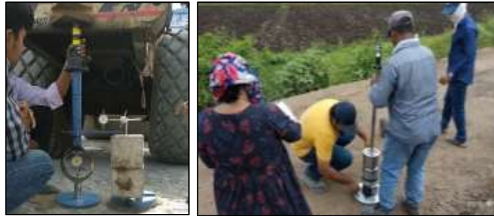
Fig. 2. Quality control testing during construction: Field CBR test (left) and LWD test (right)
