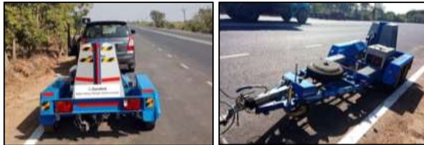
Fig. 3. Performance of FWD testing on the constructed test sections
