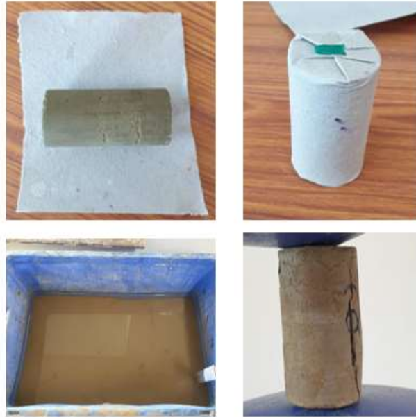
Fig. 3. Sample preparation for wetting and drying process
