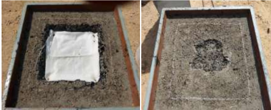
Fig 7. Pot hole simulation with and without Geotextile Layer
