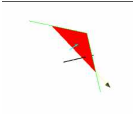
Fig. 4. Typical unstable rock wedge analyzed in SWedge software
