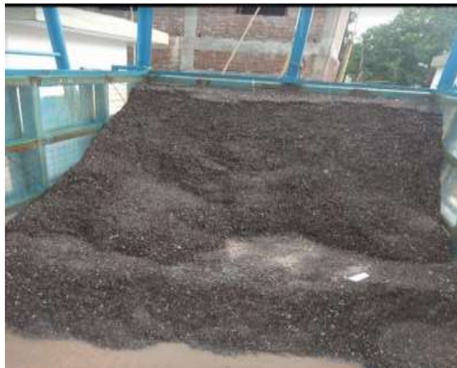
Fig.3. Slope at failure
