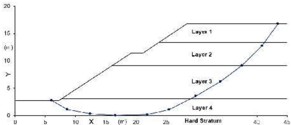
Fig. 3. Critical Slip Surface by Spencer Method for Example 1 ( $K_h = 0.10$ ).
