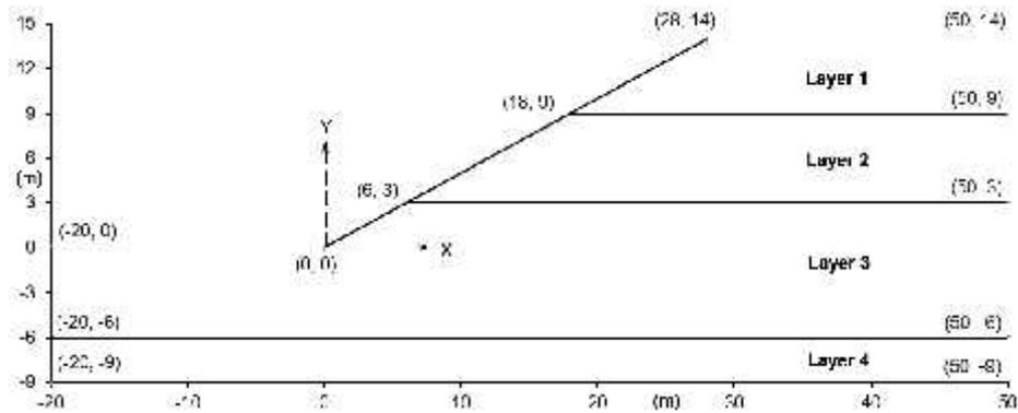
**Fig. 4.** Slope Section in Example 2 [Similar to the Slope section in Zhu and Lee (2002)].**Table 3.** Soil Properties for Example 2 [Zhu and Lee (2002)]
