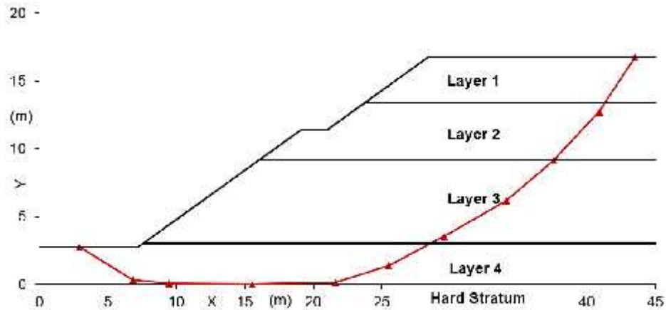
Fig. 2. Critical Slip Surface by Morgenstern and Price Method for Example 1 ( $K_h = 0.10$ )
