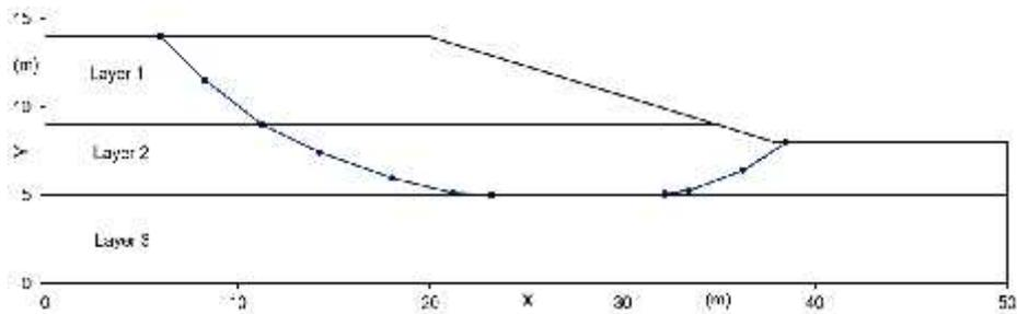
Fig. 10. Critical Slip Surface by Spencer Method for Example 3 ( $K_h=0.10$ )
