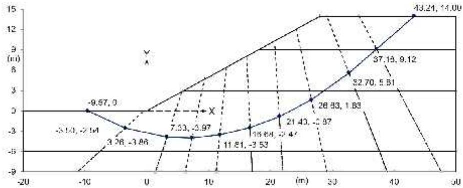
**Fig. 7(b).** Slice configuration in Sarma method of analysis of the critical slip surface based on Spencer method
