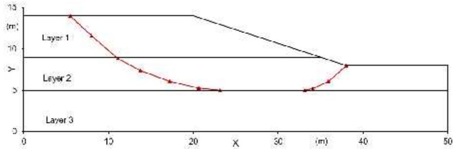
Fig. 9. Critical Slip Surface by Morgenstern & Price Method for Example 3 ( $K_h=0.10$ )
