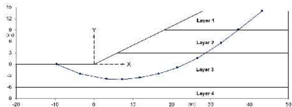
Fig. 6. Critical Slip Surface by Spencer Method for Example 2 ( $K_h = 0.20$ )
