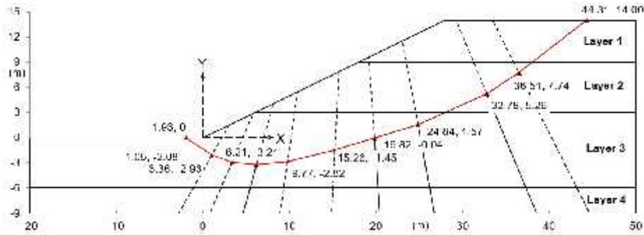
**Fig. 7(a).** Slice configuration in Sarma method of analysis of the critical slip surface based on Morgenstern and Price method
