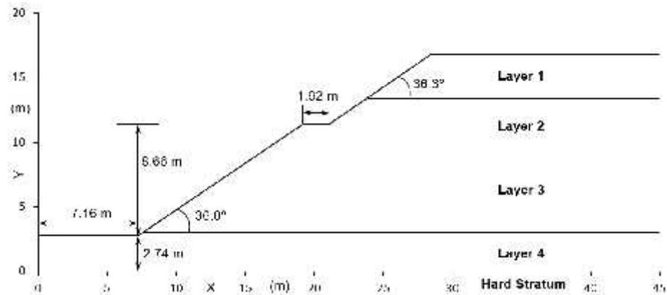
**Fig. 1.** Slope Section for Example 1: Cross-section of the Congress Street open cut [after Ji and Low (2012)].
