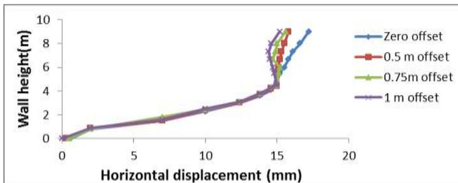
**Fig 7.** Wall deformation for different offsets of two-tiered walls subjected to Kobe earthquake excitations.
