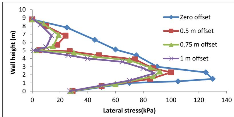
Fig.10. Lateral soil pressure on the face of the wall for different offset of two-tiered walls
