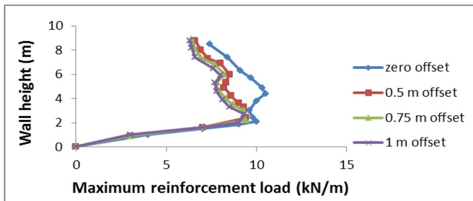
**Fig 8.** Maximum reinforcement load for different offsets of two-tiered walls subjected to Kobe earthquake excitations.
