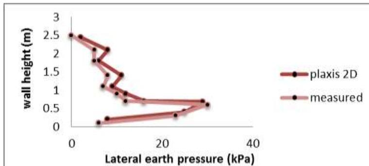
Fig 4. Predicted and measured lateral stresses of backfill at the wall face
