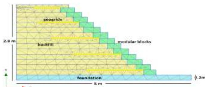
**Fig 2.** Numerical model used for validation
