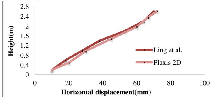
Fig 3. Horizontal displacement measured by Ling et. al.(2005) and FE analysis
