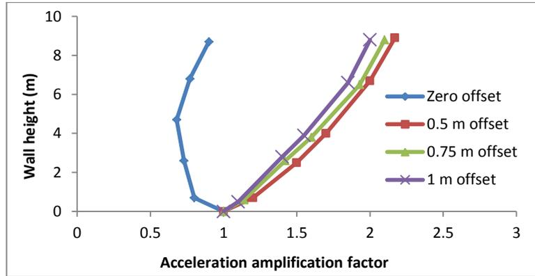
Fig.9. Horizontal acceleration amplifications in the backfill for two-tiered walls subjected to Kobe earthquake excitations.
