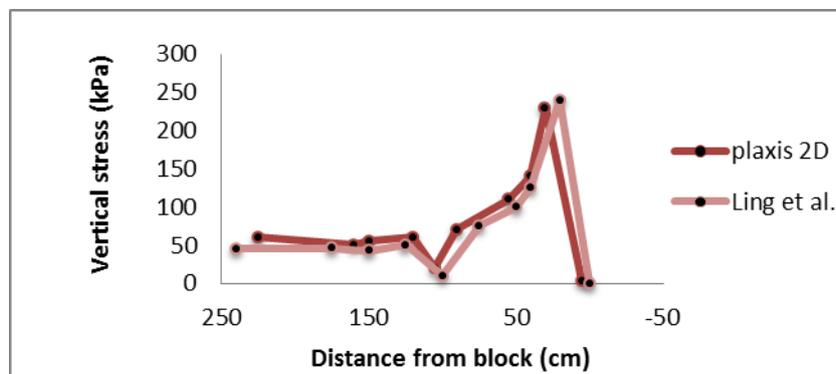
Fig 5. Predicted and measured vertical stresses at the wall base.
