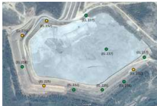
Fig.6. Approximate Location of Boreholes on Google Image
