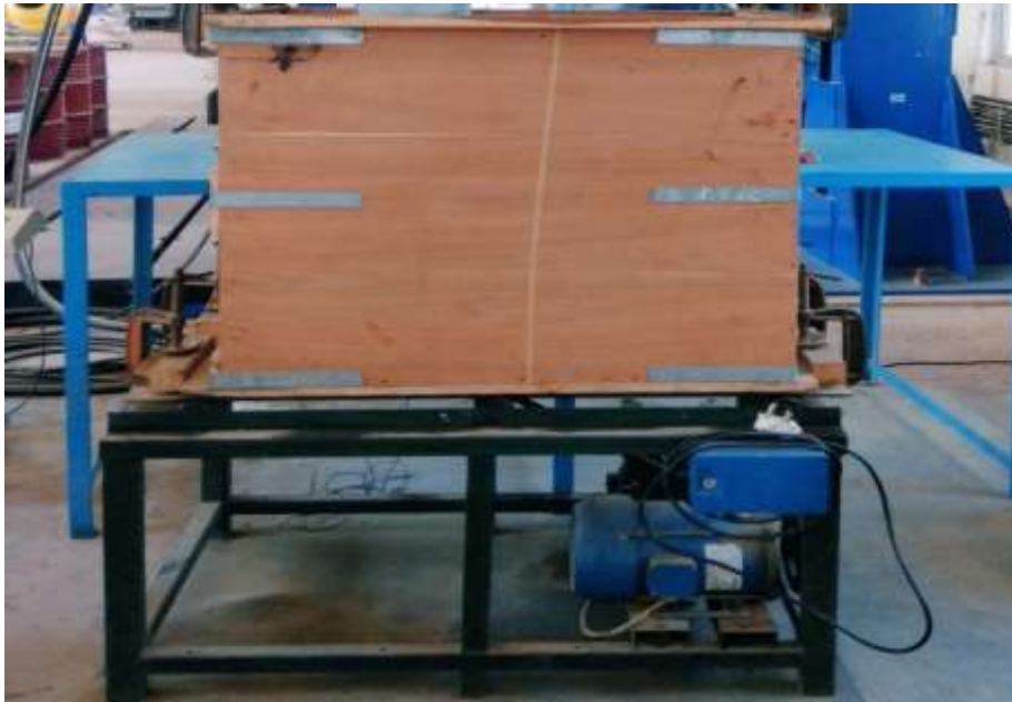
Fig. 1. The seismic box mounted on the shake table.
