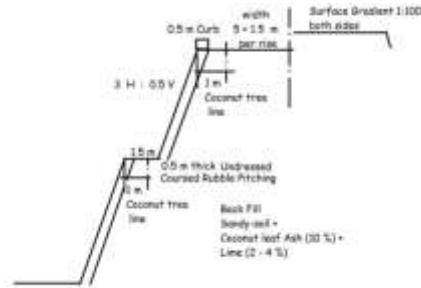
Fig. 7. Typical Dimensions of Traditional Goan Saraswat Bunds
