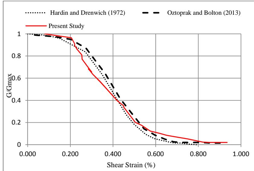
**Fig. 3.** Variation of  $G/G_{max}$  with Shear Strain and comparison with past experimental results.
