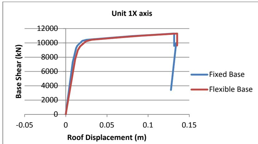
**Fig 7.1:** Pushover Capacity curves for Fixed and Flexible base foundations for Unit 1 for X axis loading.
