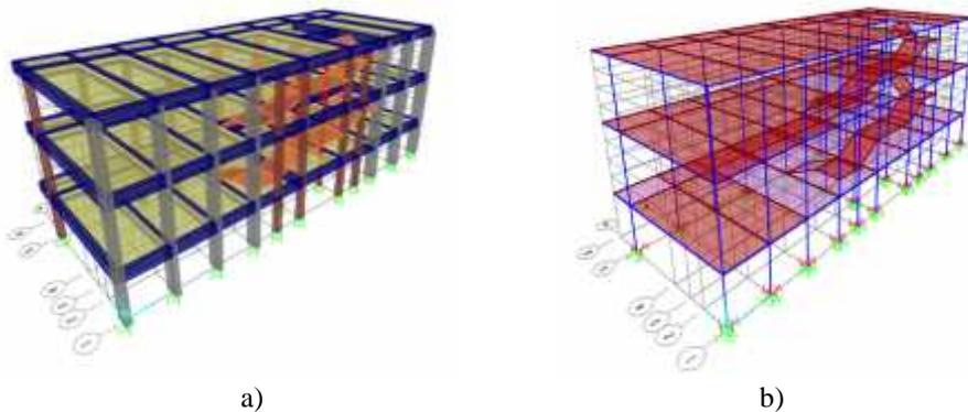
**Fig 6.2:** Unit 7 modelled with Fixed and Flexible base Foundations: a) Fixed Base Model and b) Flexible Base Model (springs are assigned).
