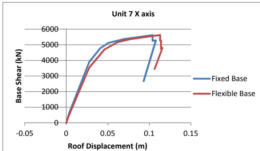
**Fig 7.2:** Pushover Capacity curves for Fixed and Flexible base foundations for Unit 7, for X axis loading.
