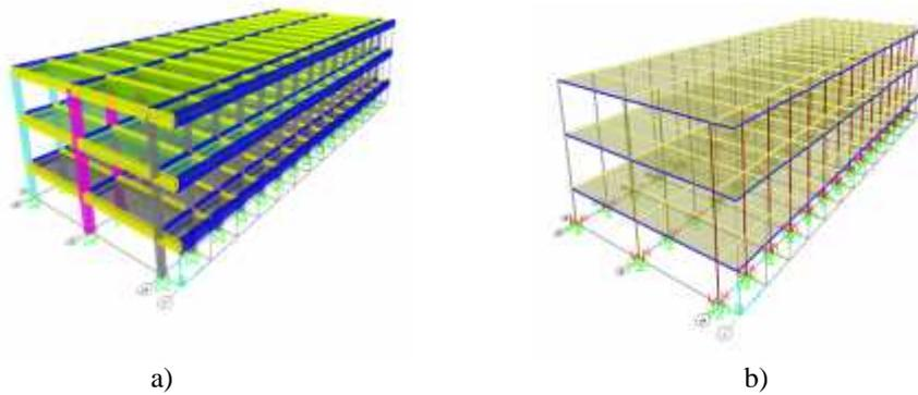
**Fig 6.1:** Unit 1 modelled with Fixed and Flexible base Foundations: a) Fixed Base Model and b) Flexible Base Model (springs are assigned).
