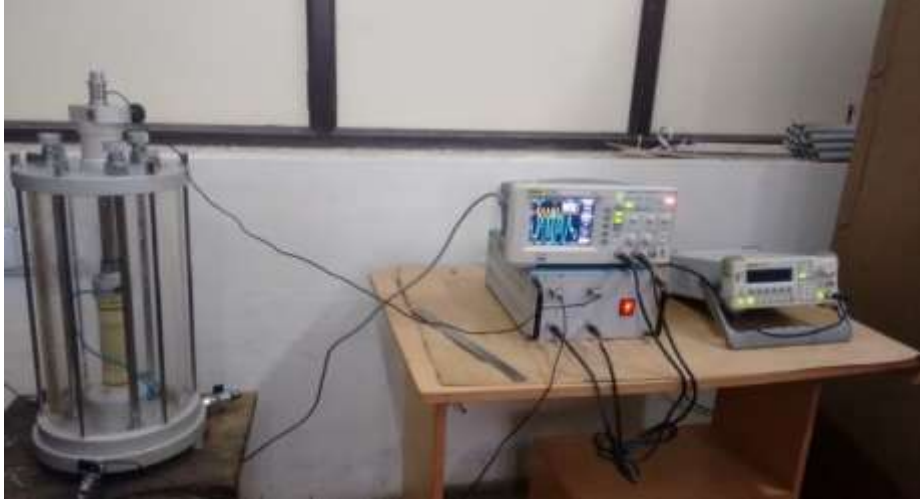
Fig. 2. Bender element test on cemented specimen
