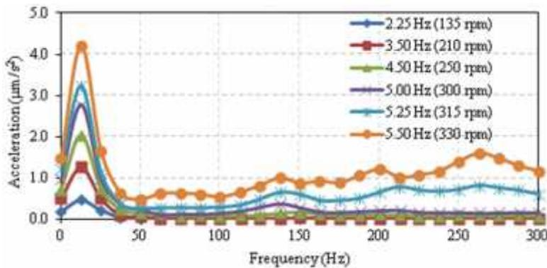
**Fig. 11.** Influence of frequency on response of UGSM layer at 20 mm from base
