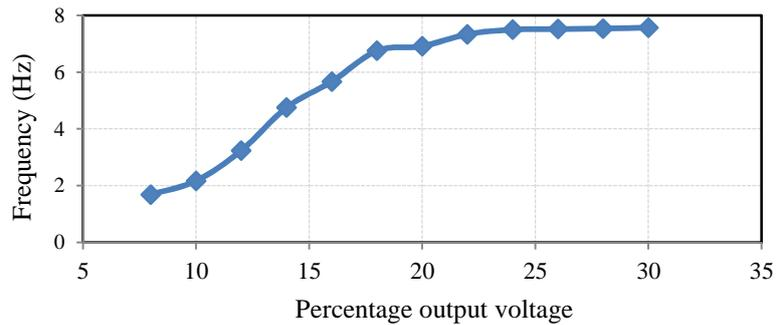
**Fig. 3.**Calibration of VARIAC against frequency using Tachometer
