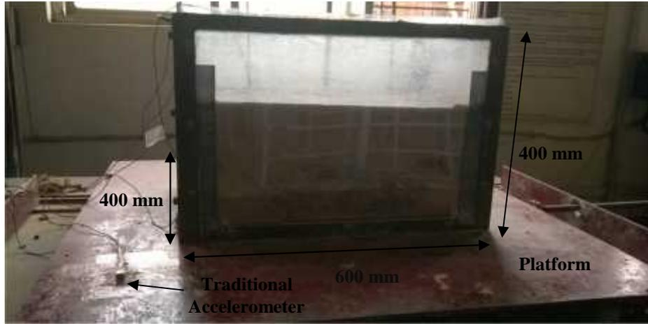
**Fig. 2.** Soil model container monolithically attached with shake table
