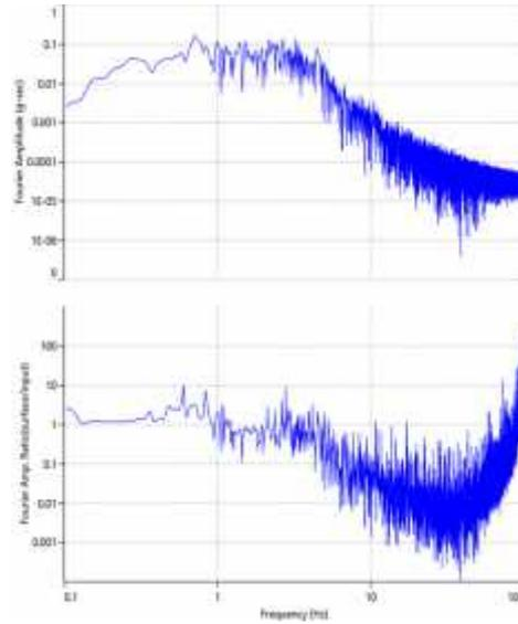
**Fig. 15.** Fourier amplitude spectrum of surface layer of USC
