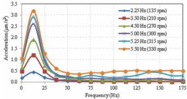
**Fig. 12.** Influence of frequency on response of UGSM layer at 50 mm from base
