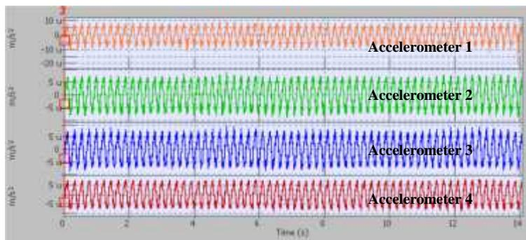
**Fig. 4.**Typical acceleration time history of UGSM at 4.50 Hz
