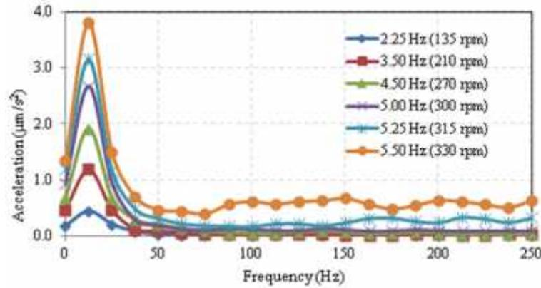
**Fig. 13.** Influence of frequency on response of UGSM layer at 70 mm from base
