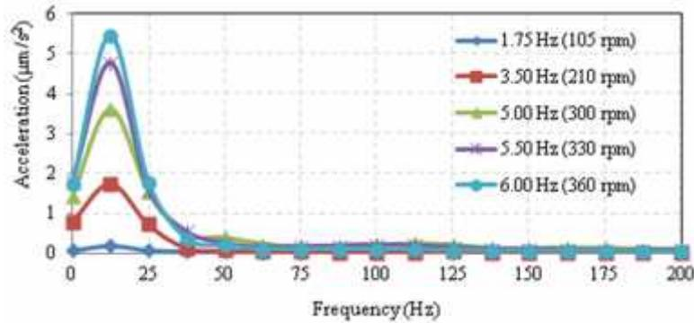
**Fig. 10.** Influence of frequency on response of USSM layer at 200 mm from base
