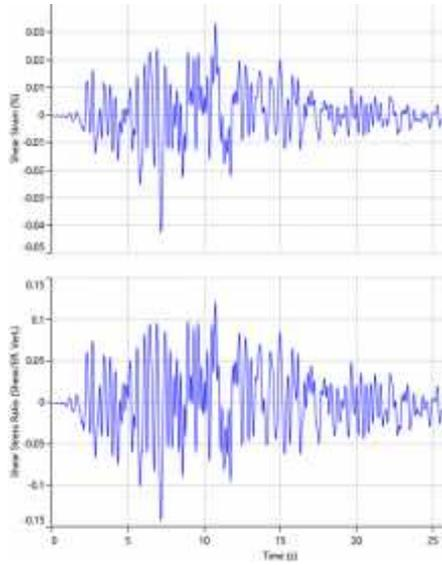
**Fig. 14.** Shear strain and shear stress ratio at surface layer of USCM
