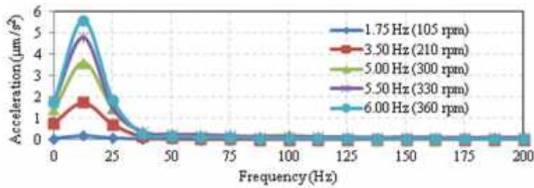
**Fig. 8.** Influence of frequency on response of USSM layer at 10 mm from base
