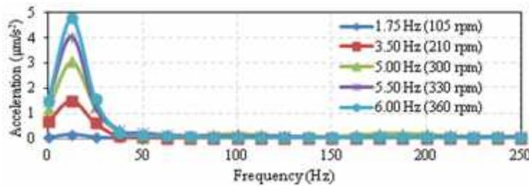
**Fig. 9.** Influence of frequency on response of USSM layer at 100 mm from base
