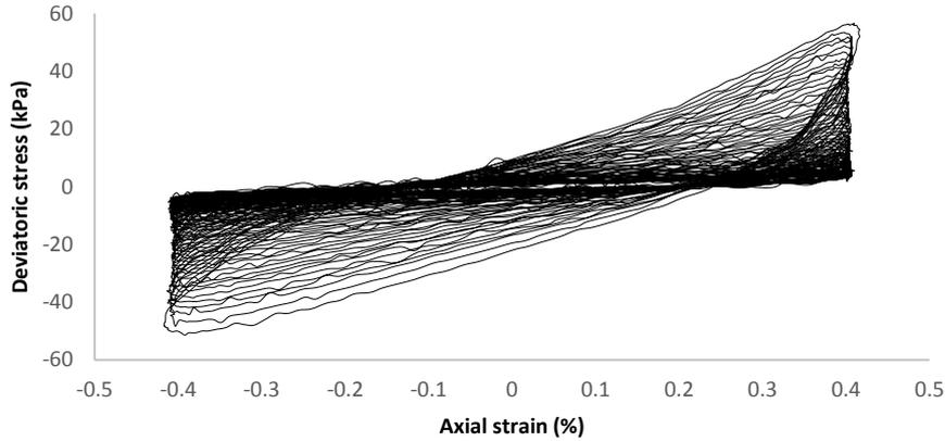
**Fig. 3.** Variation of deviatoric stress with axial strain (hysteresis loop) for 100 mm diameter pond ash sample at 50 kPa confining pressure and 0.4% strain rate.
