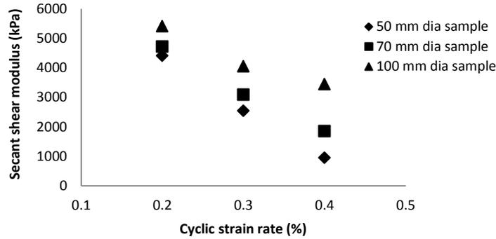
**Fig. 5.** Effect of sample size and strain rate on secant shear modulus of Panki pond ash samples tested at 50 kPa confining pressure and 1 Hz loading frequency.
