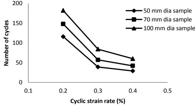
**Fig. 4.** Effect of sample size and strain rate on liquefaction resistance of Panki pond ash samples tested at 1 Hz loading frequency.
