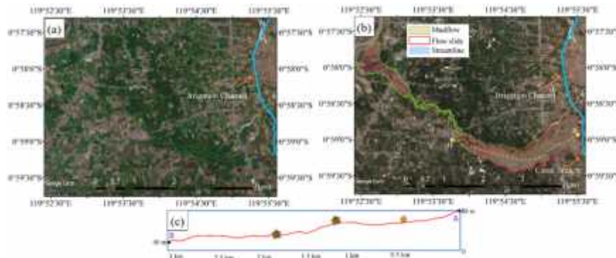
Figure 3: Lateral flow area in Juno Oge village due to Sulawesi Earthquake, (a) before flow failure, (b) after flow failure with mud flow and water channel and (c) slope profile of the flow area (modified from Google Earth).
