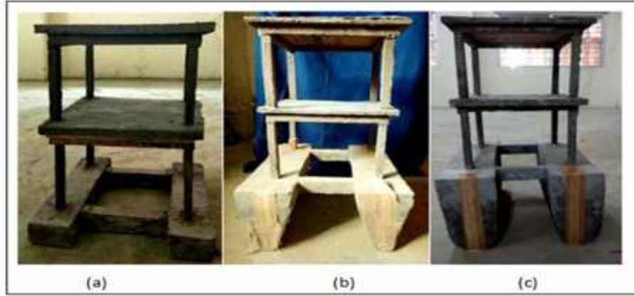
Figure 1. Pictorial view of (a) rectangular (b) trapezoidal and (c) bowl shaped footing.
