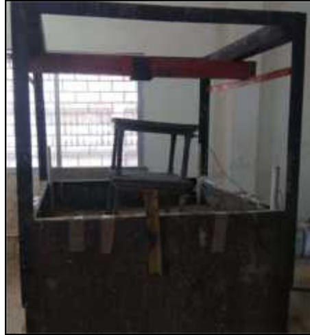
Figure 14. Tilt of rectangular shaped building frame after shaking.
