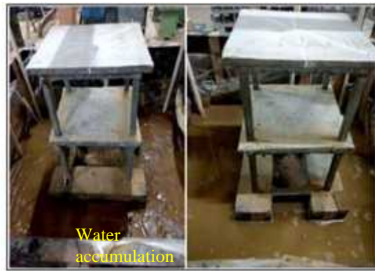
Figure 13. Building on bowl shaped footing before and after liquefaction.
