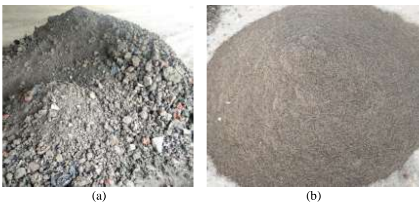
Fig. 2. (a) Stockpile of MSWI bottom ash, (b) Soil-like-fraction from MSWI bottom ash
