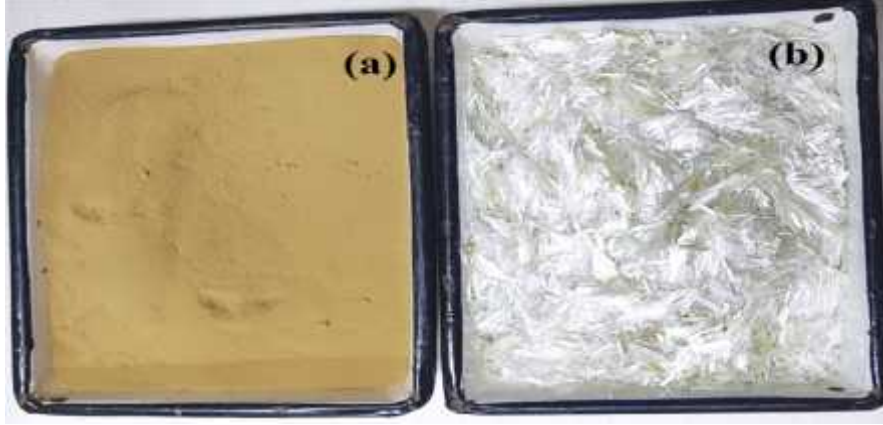
Fig. 1. Photograph of the materials used in the study, (a) Mixture clay, (b) Glass fiber
