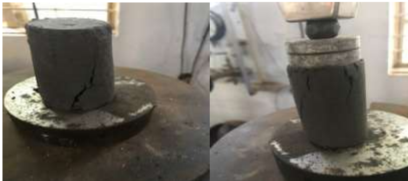
Fig 3. Stress-strain behaviour of lime stabilized coal gangue
