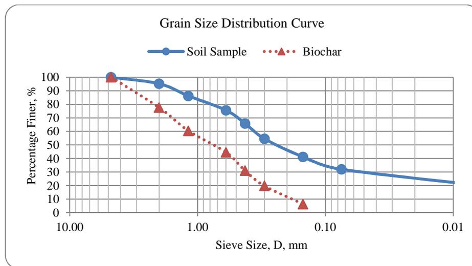
**Fig.7.** Grain Size Distribution Curve of Soil sample and Biochar
