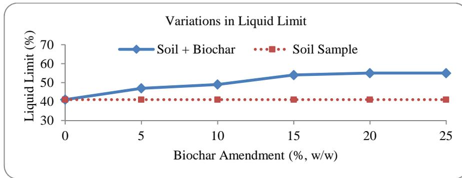
**Fig.8.** Effect of Biochar Amendment on Liquid Limit of Soil
