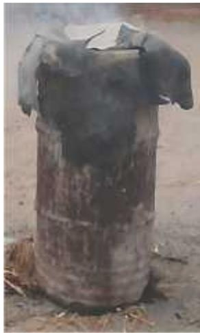
**Fig.5.** Drum covered after initial burning & kept for 15 min for pyrolysis
