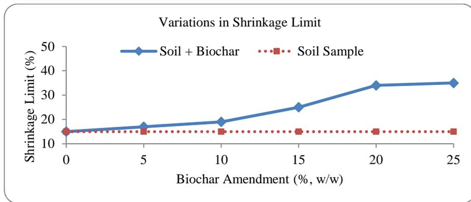
**Fig.10.** Effect of Biochar Amendment on Shrinkage Limit of Soil
