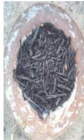
**Fig.6.** Biochar produced by pyrolysis
