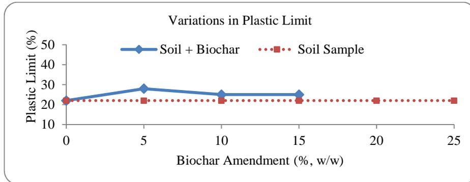
**Fig.9.** Effect of Biochar Amendment on Plastic Limit of Soil
