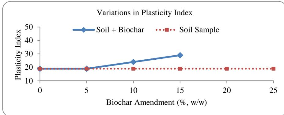
**Fig.11.** Effect of Biochar Amendment on Plasticity Index of Soil
