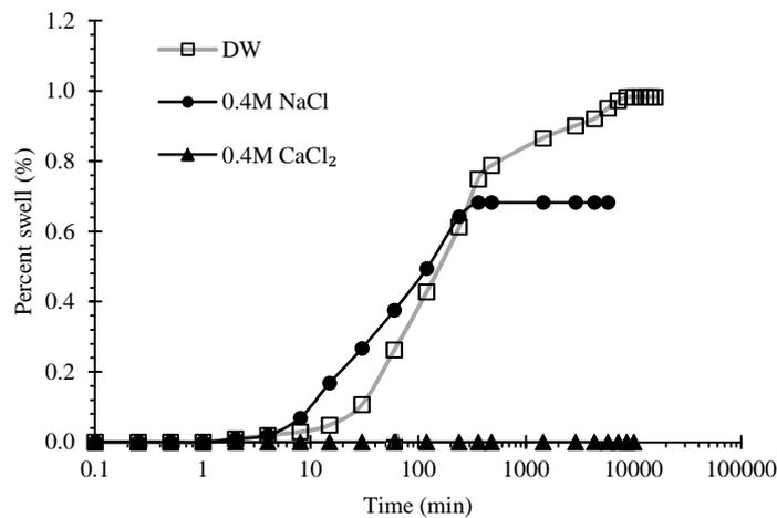
**Fig. 5. a.** Effect of salt concentration on time-swell plots of compacted red soil-bentonite specimen B1
