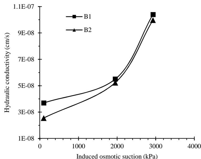
**Fig. 6. b.** Effect of induced osmotic suction on hydraulic conductivity of red soil-bentonite mixtures
