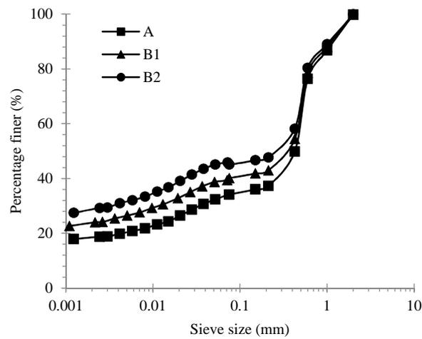
**Fig. 1.** Grain size distribution curves
