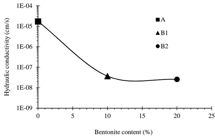
**Fig. 4.** Effect of bentonite content on hydraulic conductivity of red soil using distilled water as inundating fluid
