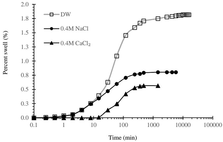
**Fig. 5. b.** Effect of salt concentration on time-swell plots of compacted red soil-bentonite specimen B2
