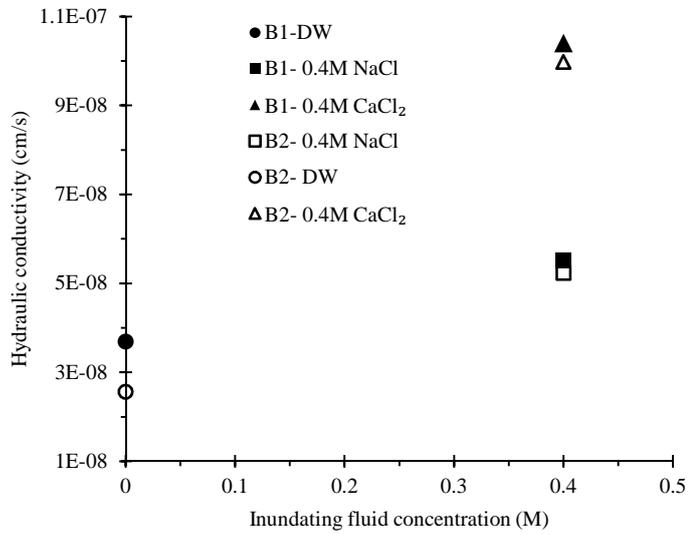
**Fig. 6. a.** Variation of hydraulic conductivity with inundating fluid concentration
