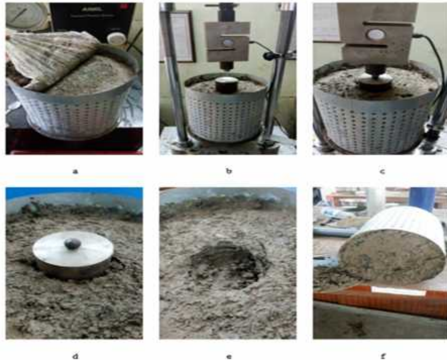
Fig. 6. Testing procedure (a) Removing top cover after soaked for 96 hours, (b) Placing mould under loading frame along with footing at centre, (c) Applying point load to the footing, (d) Footing after testing, (e) Settlement of the footing, (f) Removing sample from the mould
