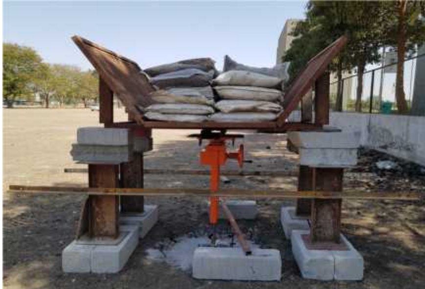
Fig 7. Plate load test using Geo-cell
