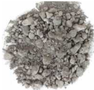
Fig.1 Visual appearance of steel slag
