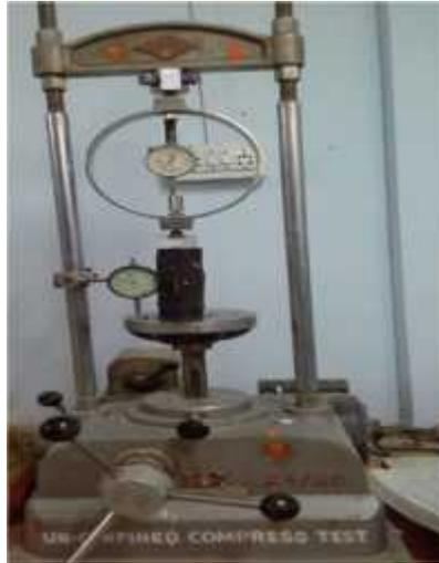
Fig. 7. Test setup used for the UCS test
