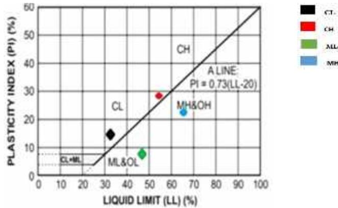
**Fig. 1.** Location of the used samples in soil plasticity chart
