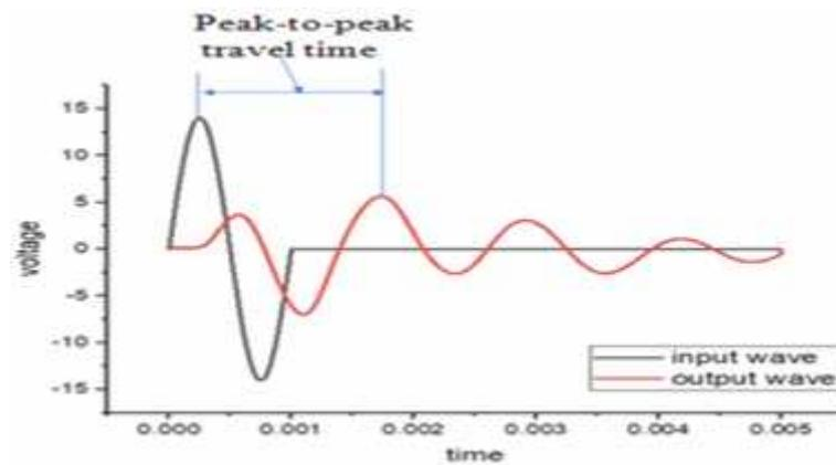
Fig. 6. Determination of peak-to-peak travel time
