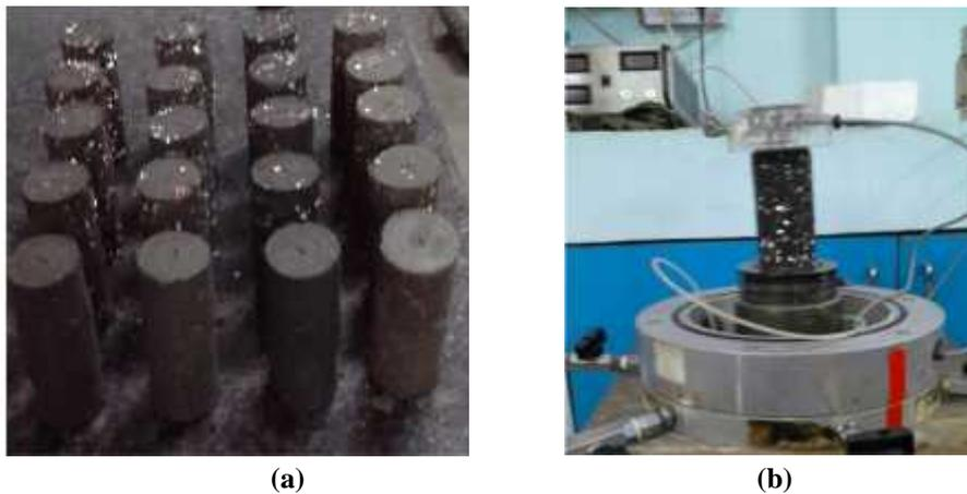
**Fig. 4.** (a) Soil samples used for the bender/extender testing (b) Bender/Extender test.
