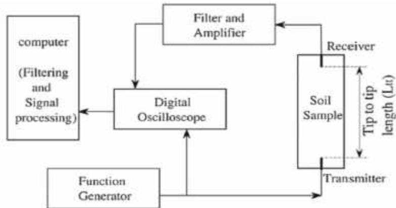
Fig. 5. Schematic representation of bender/extender test setup
