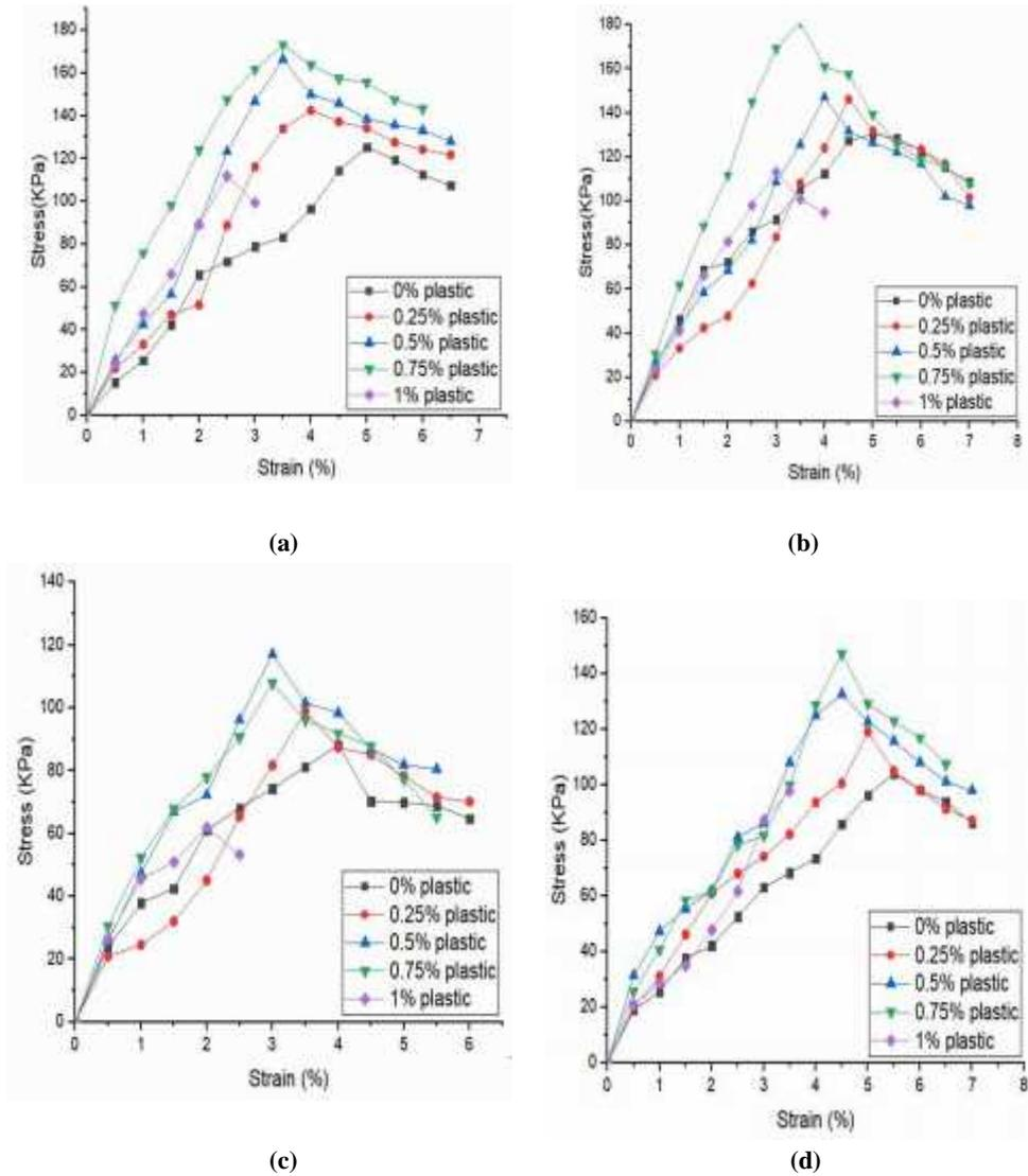
**Fig. 11.** Stress-strain curves obtained from UCS tests for (a) CL (b) CH (c) ML (d) MH soils
