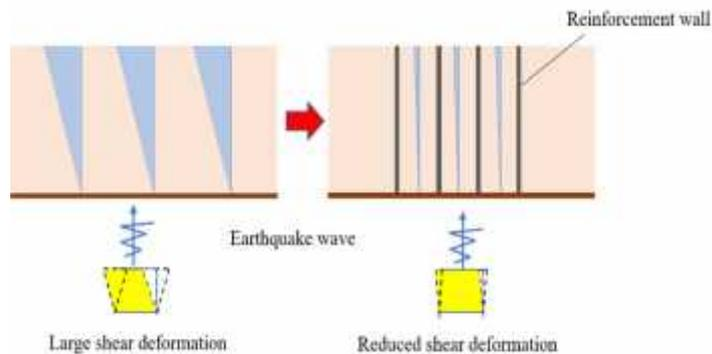
**Fig. 1.** Liquefaction mitigation mechanism of grid form wall
