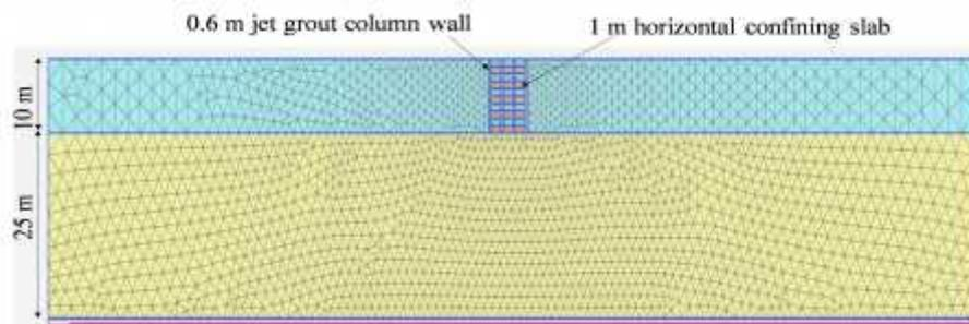
**Fig. 4.** Finite element model of the improved case
