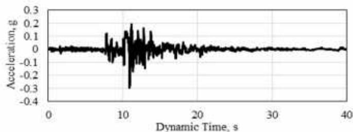
**Fig. 2.** Seismic Input motion applied in the Analyses
