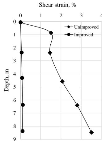
**Fig. 8.** Distribution of shear strain in unimproved and improved cases with depth
