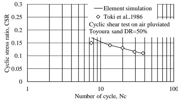
**Fig. 3.** CSR ratio obtained from numerical and experimental results
