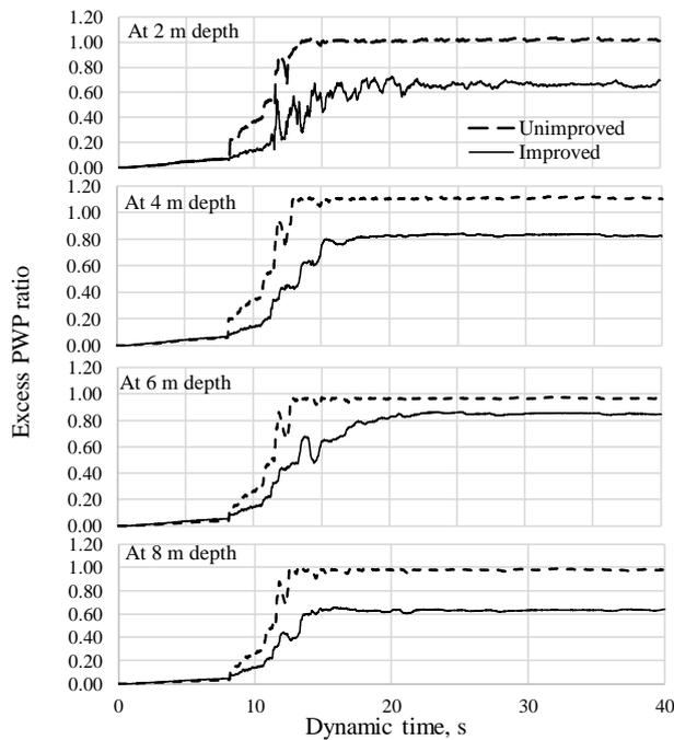
**Fig. 5.** Comparison result of PWP ratio measured from unimproved and improved cases
