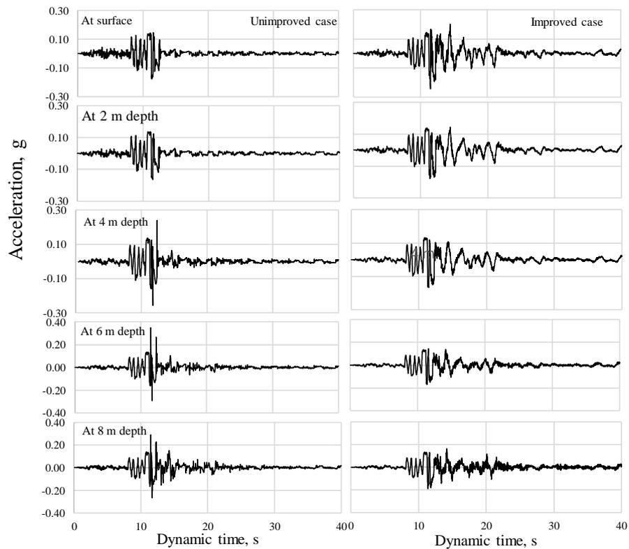
**Fig. 6.** Acceleration time histories measured from unimproved and improved cases
