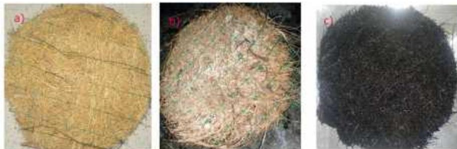
**Fig. 4.** Normal coir (NC); b) Lime Coir (LC); c) Silica Coir (SC)
