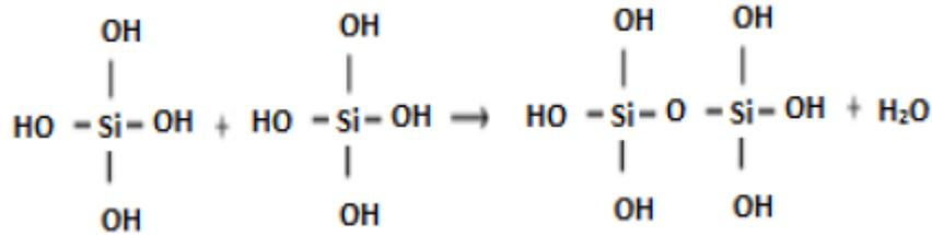
**Fig. 2.** Illustration of siloxane bonding [18].
