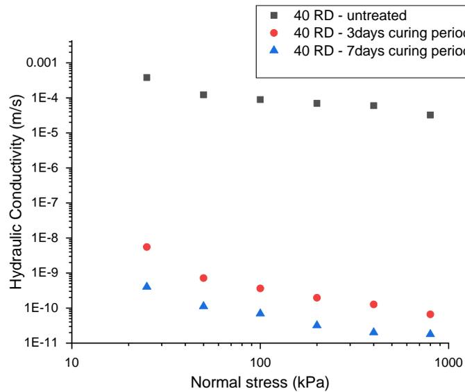
**Fig 8.** Hydraulic conductivity of untreated as well as colloidal silica treated samples at a relative density of 40 RD: Curing periods of three days and seven days
