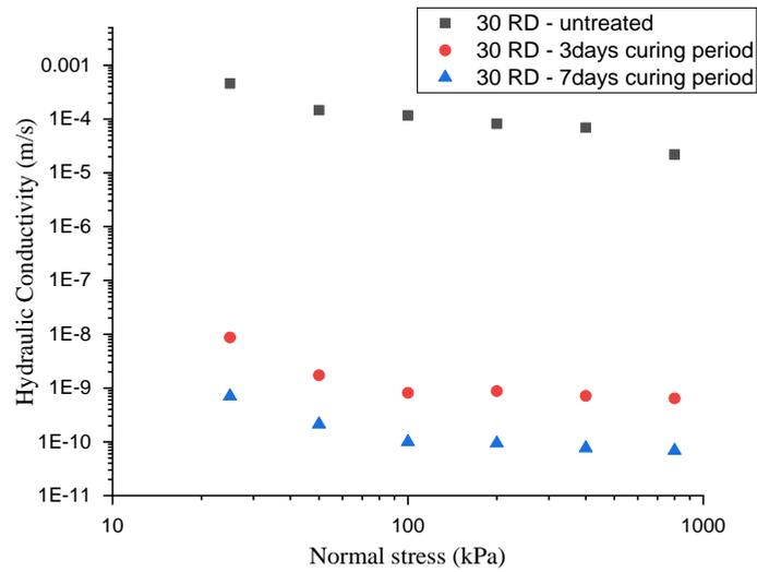
**Fig 7.** Hydraulic conductivity of untreated as well as colloidal silica treated samples at a relative density of 30 RD: Curing periods of three days and seven days
