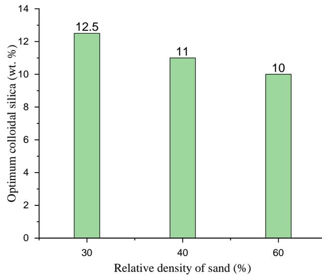
**Fig 4.** Optimum colloidal silica content for sand samples at three different densities
