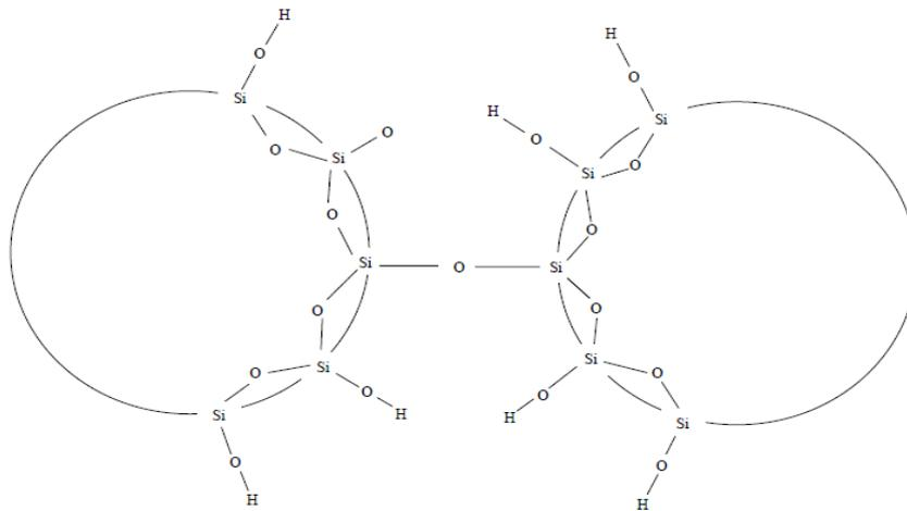
**Fig. 3.** Siloxane bond formation during gelation of colloidal silica particles [21]
