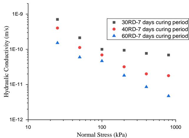
**Fig 6.** Hydraulic conductivity of colloidal silica treated samples at three different relative densities: Curing period of seven days
