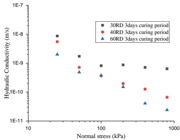
**Fig 5.** Hydraulic conductivity of colloidal silica treated samples at three different relative densities: Curing period of three days
