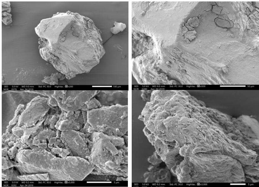
**Fig 10.** SEM images of Sand treated with colloidal silica
