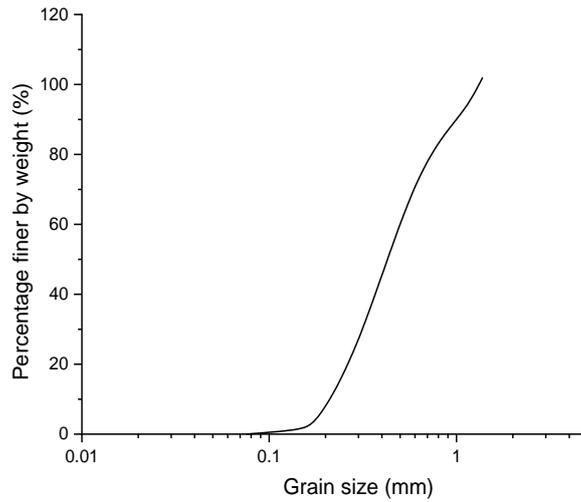
**Fig. 1.** Grain size distribution curve of untreated sand
