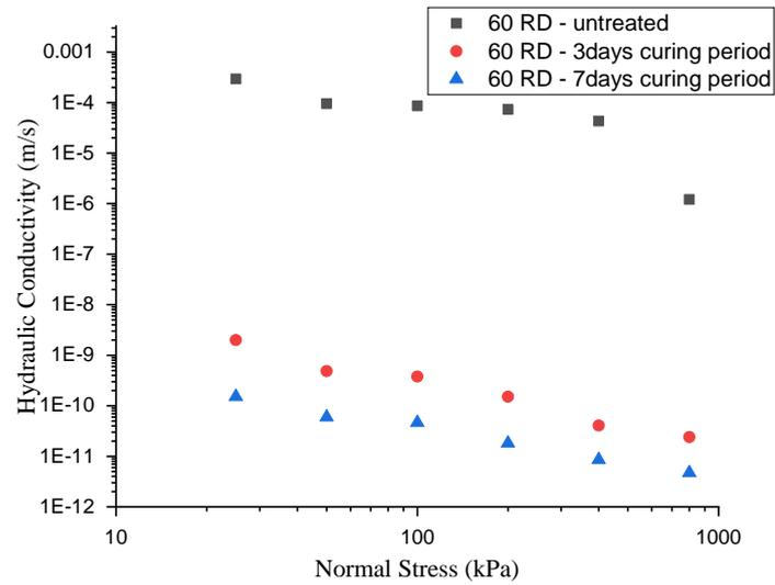
**Fig 9.** Hydraulic conductivity of untreated as well as colloidal silica treated samples at a relative density of 60 RD: Curing periods of three days and seven days
