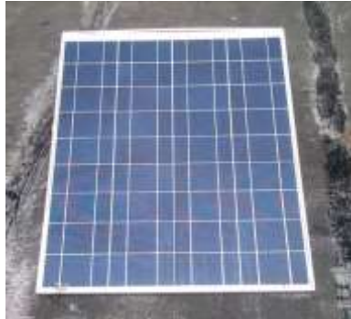
Fig. 1. View of Solar panel – 50 Watts (Size 900mm X660mm)
