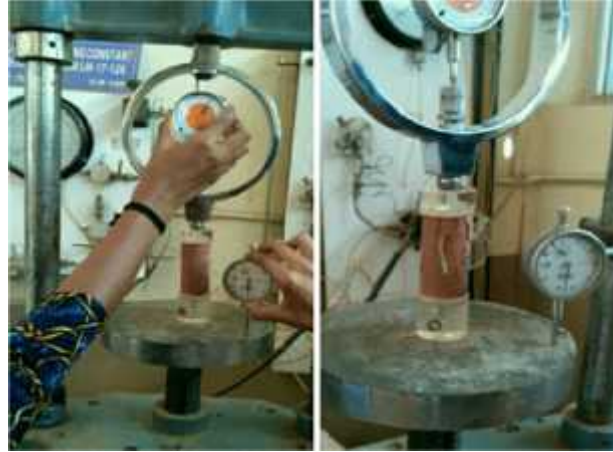
Fig. 5. The UCS tested sample before and after failure.
