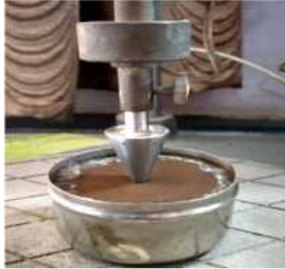
Fig. 1 Experimental setup for fall cone test
