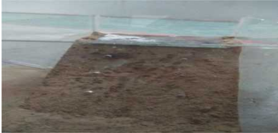
Fig 1.0. Model box with 45^\circ soils and with nails for test.
