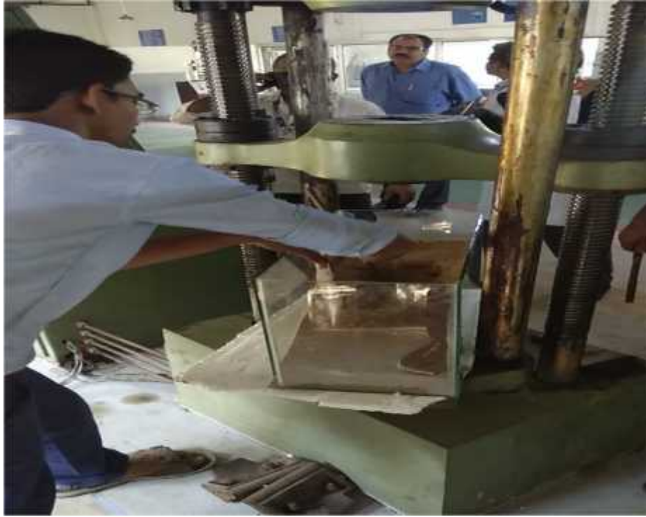
Fig 2.0. Model box under load test.
