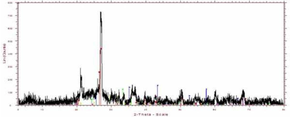
Figure 1 XRD pattern of Class F fly ash used in the study
