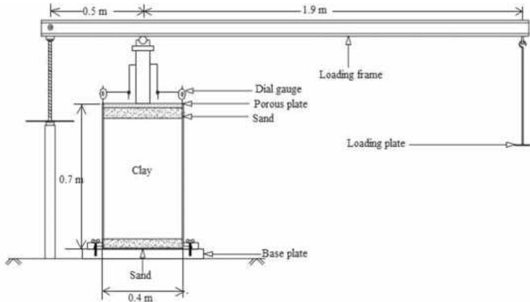
Figure 2 Arrangement of column in the model tank
