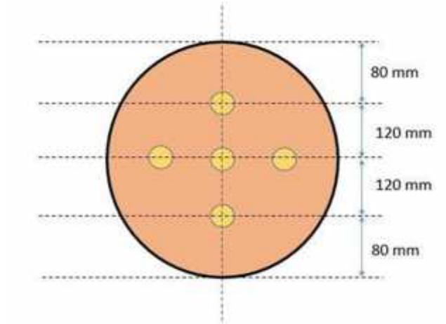
Figure 3 Arrangement of column in the model tank
