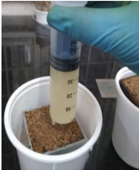
Fig. 2. Injection of Solutions into the Specimens
