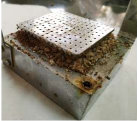
Fig. 3. MICP Treated Specimen after Shearing
