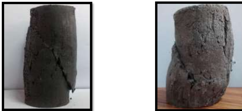
Fig. 7. Failure pattern of unreinforced and reinforced soil
