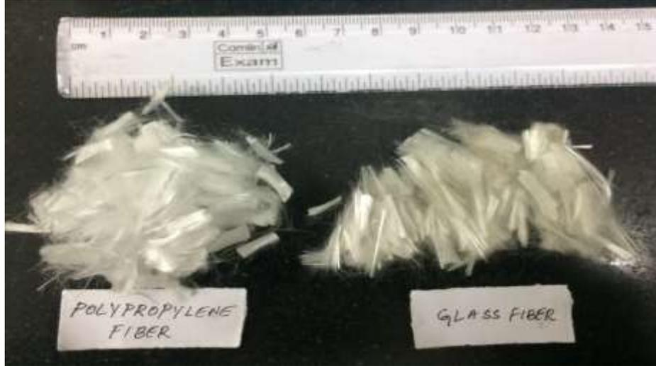
**Fig. 2.** Image showing discrete Polypropylene and Glass fiber
