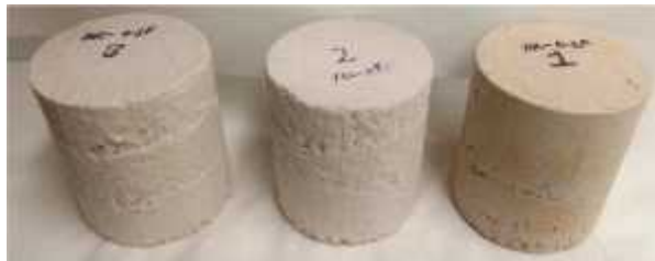
Fig. 6. Sample stabilized with 10% cement and 0.5% fiber after 12 weathering cycle
