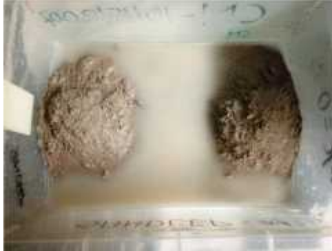
Fig. 5. EPK clay sample collapsed during wetting stage of 2 nd cycle
