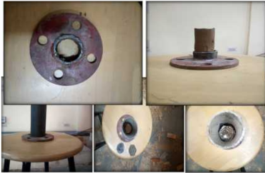
Fig 2 Mould and sample preparation for curing stress
