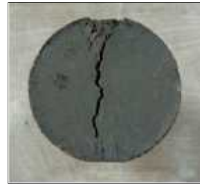
Fig. 6. Failure pattern of specimen in STS test
