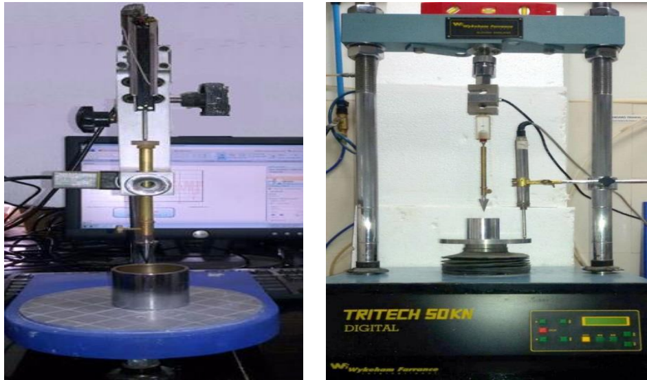
Fig. 1. a) Modified fall cone apparatus b) Cone connected to the loading frame.
