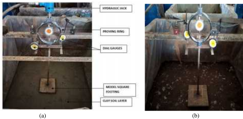
Figure 3. (a) Model tank with loading arrangement on soft clay layer (b) Placing the cement modified fibre reinforced sand layer on top of soft clay layer
