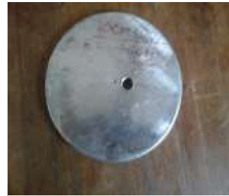
Fig. 3. Model Circular footing
