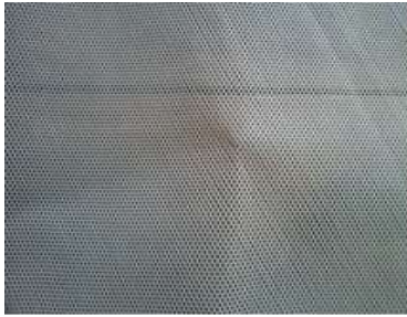
Fig. 2. Typical Geonet material
